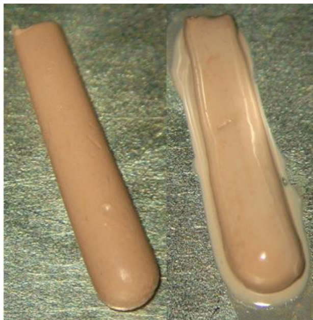
Figure 1 - Gutta-percha point standardized at 10 mm before and after the solvent application
